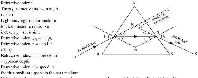
Refractive index of a triangular glass prism, can be expressed as: n =  $\{\sin \frac{1}{2} (A + D_{min})\} / (\sin \frac{1}{2} A) A = 2r, D_{min} = 2i - 2r^*$
