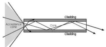
There are two main types of optical fibres: mono-mode and multimode. Mode means a form of bandwidth or frequency,
