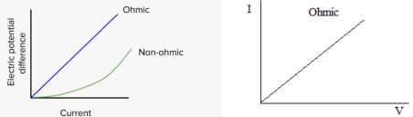
Differentiating between Ohmic and Non-Ohmic conductor
